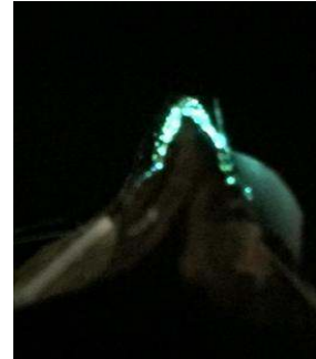
Flexible green InGaN/GaN NW LED
