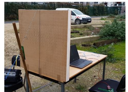
Figure 1. Focusing metasurface device setup
